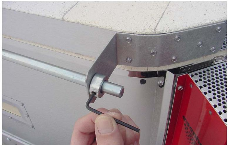
Center the Dyna-Lift link on the lid handle rod. Once centered move the collar clamps up to each side of the link and tighten with the 1/8" allen wrench.
