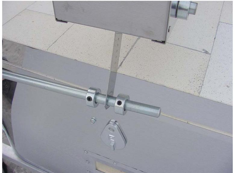
Re-insert the lid handle rod into the right side lid bracket. Place the collar clamp on the end of the lid handle rod and tighten with the allen wrench.
