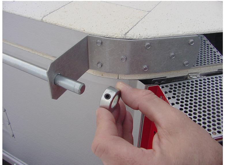
Pull the lid rod out of the right lid bracket until its end is roughly at the mid-point of the kiln. Place 1 collar clamp onto the lid rod. Extra collar clamps are included in the parts package.
