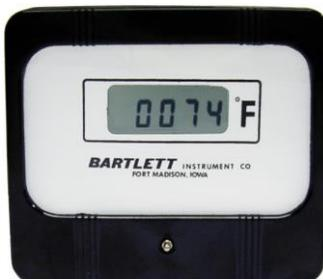
A pyrometer is a meter used to measure the temperature in side the kiln. A thermocouple (sensing probe) is attached to the meter and is inserted 1-1/2” to 2” (4 to 5cm) into the kiln chamber.
