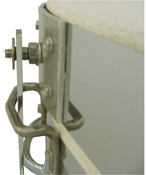
Install the nut on the pin and tighten.
