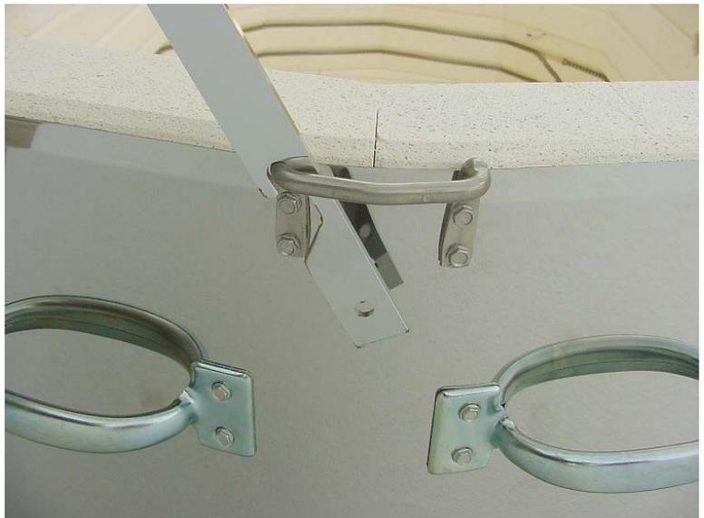
Remove the nut and bushing from the pin mount. Place the upper hole of the lid security bar on the pin mount located on the lid. Install the bushing on the pin and tighten. Install the bushing so it sinks into the hole on the security lid bar. This allows the bar to move against the bushing and not the pin threads.
